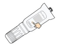
Figure 7-2 Enabling the WLAN Hotspot
