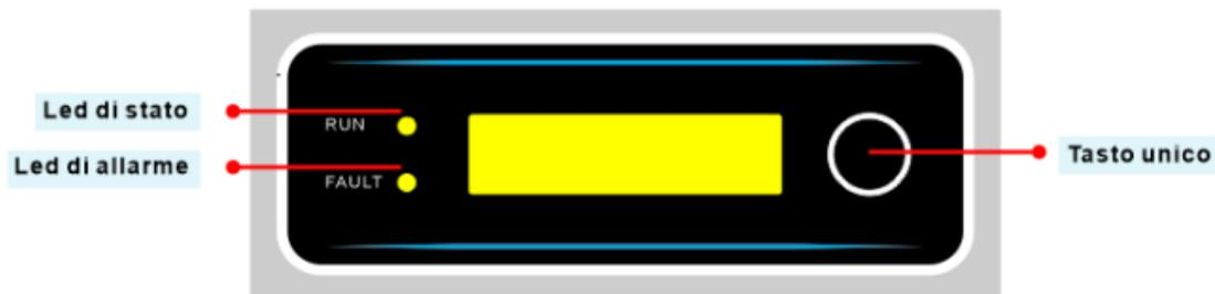
Figure 37 – LCD display with buttons and LED indicators
