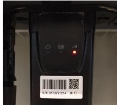
Figure 61 - Irregular communication status between Wi-Fi and remote server
