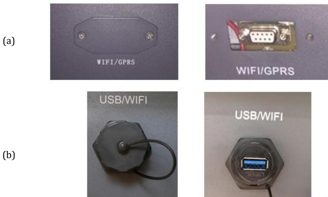
Figure 39 – Port for external Wi-Fi adapter
