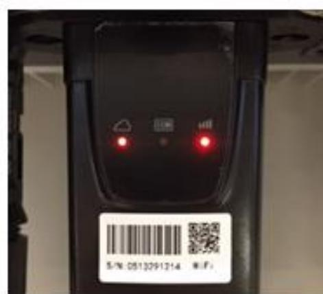
Figure 59 - Irregular communication status between inverter and Wi-Fi
