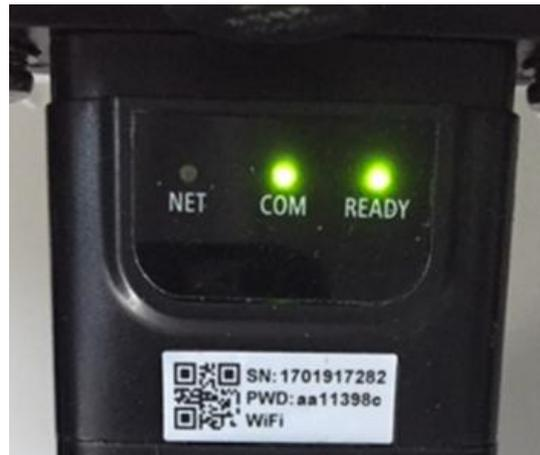
Figure 71 - Irregular communication status between the adapter and remote server
