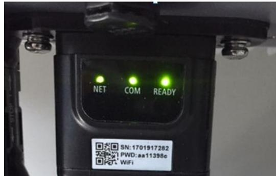
Figure 75 - Final status of LEDs
