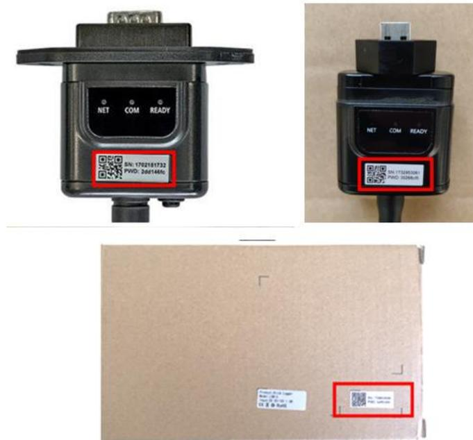
Figure 44 - Password of external Wi-Fi adapter
