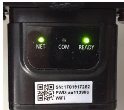
Figure 76 - Irregular communication status between inverter and adapter
