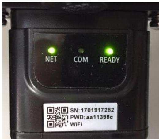
Figure 70 - Irregular communication status between the inverter and adapter
