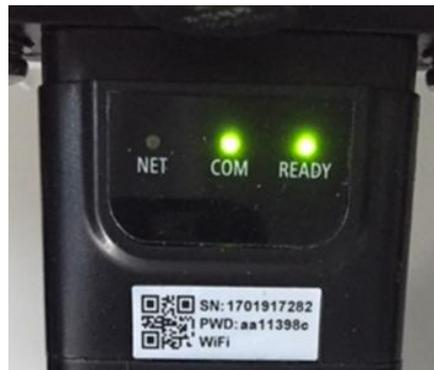
Figure 77 - Irregular communication status between the adapter and remote server
