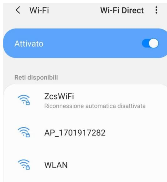
Figure 42 - Disabling automatic reconnection to a network
