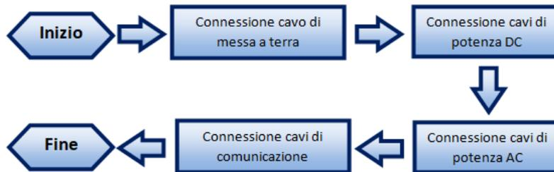
Figure 14 – Steps for connecting the cables
