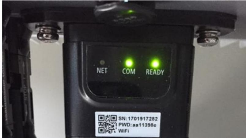
Figure 68 - Initial status of LEDs
