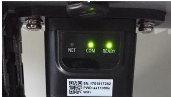
Figure 74 - Initial status of LEDs
