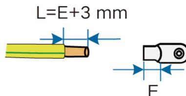
**step 3** Prepare the cable by crimping the OT/DT terminal, as shown in the below figure.
