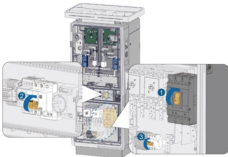
**step 3** Close the door of the charger. Check the indicators. If the top indicator is steady green, the charging connector is in standby mode; if the Energy Star-Ring is steady blue, the charger is working normally.
