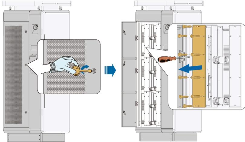
**step 3** Remove the screws and wiring terminals connected to the power unit.
