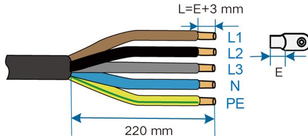
**step 6** Crimp the OT/DT terminals onto the wires by referring to the instructions shown in the figure.
