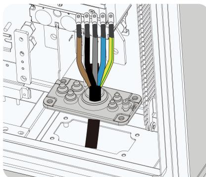
**step 8** Mount the waterproof sealing plate back on the AC cable inlet of the charger, using the screws that are removed before.
