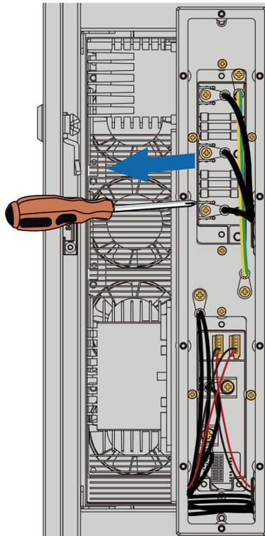
**step 4** Open the right cabinet door on the charger using the key included in the accessories. Remove the gasket used to fix the power unit. Pull the power unit out of the cabinet by its handles.
