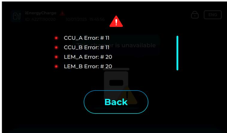
**step 2** You can tap **Back** to close the details window. By tapping the red fault icon
