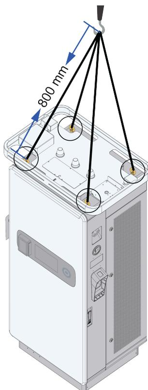
**step 2** Hoist the charger vertically and smoothly. Make sure it is always held steady and does not tilt.
