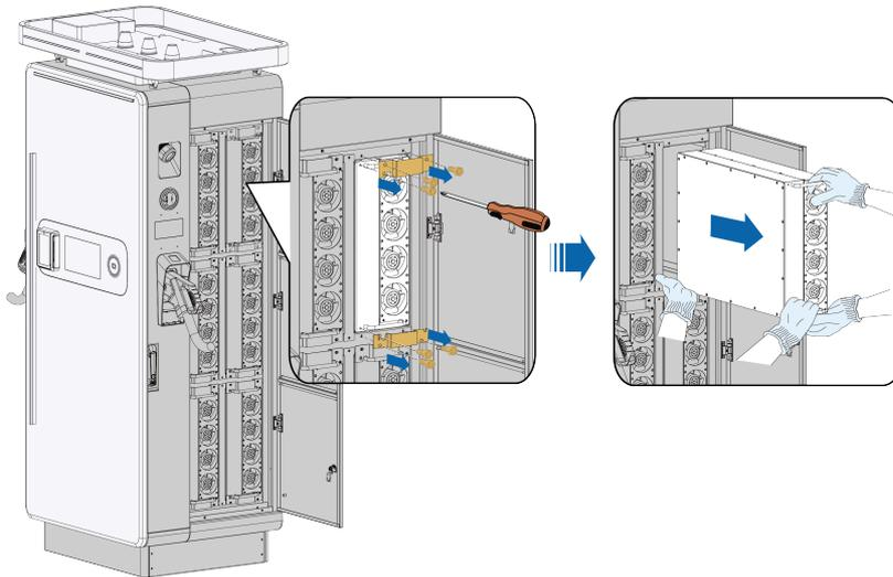
**step 5** Slowly push the new power unit into the cabinet. Fit the gasket, screws, and wiring terminals back, by performing the above steps in the reverse order.
