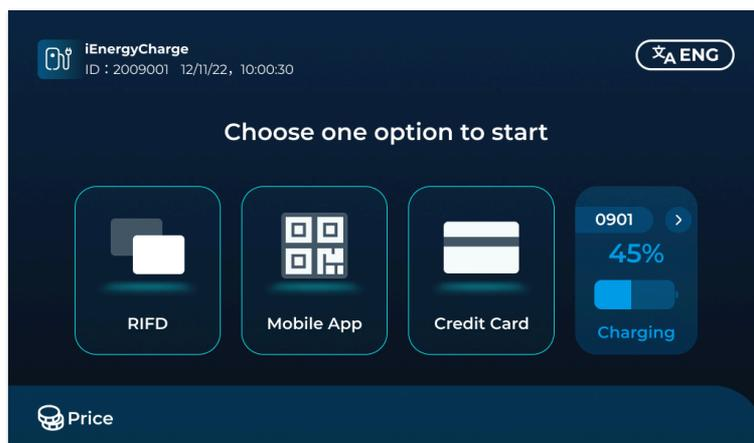
**step 10** Taking the RFID card as an example, if you choose "RFID", the Energy Star-Ring on the device will blink blue, waiting for you to tap a card over the reader. Upon detecting the card, the system
