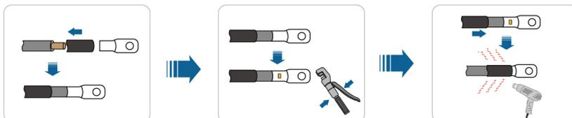
**step 4** Connect the prepared grounding cable to the grounding copper bar on the back of the charger.
