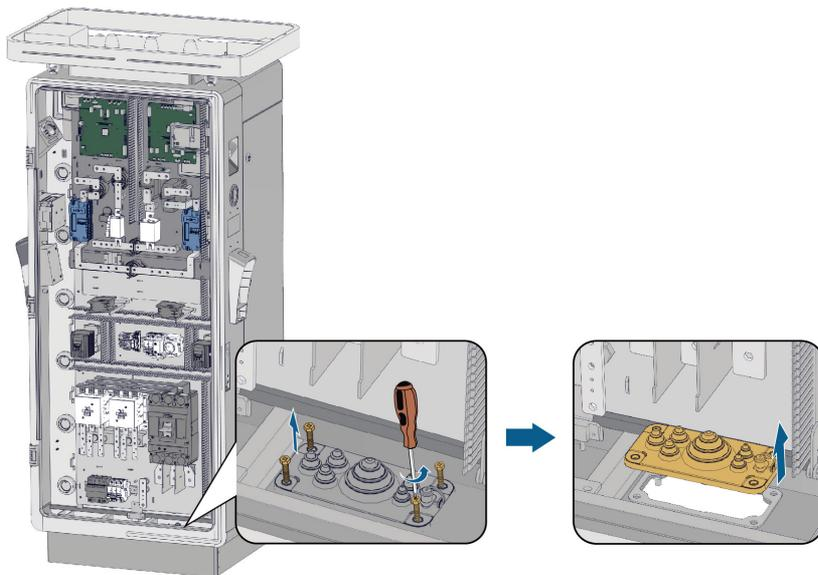
**step 4** Trim the seal to make an opening, which should be done properly according to the outer diameter of the AC cable.
