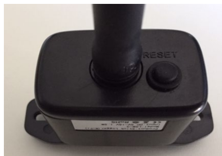
Figure 121 – Reset button on the Wi-Fi adapter
