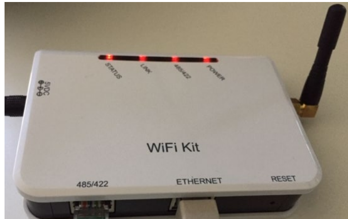
Figure 164 – LED indicating the correct configuration of the datalogger
