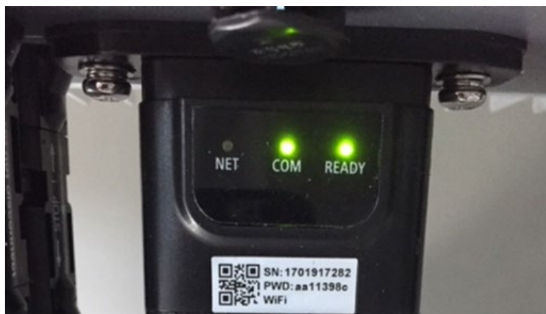
Figure 131 – Initial status of LEDs
