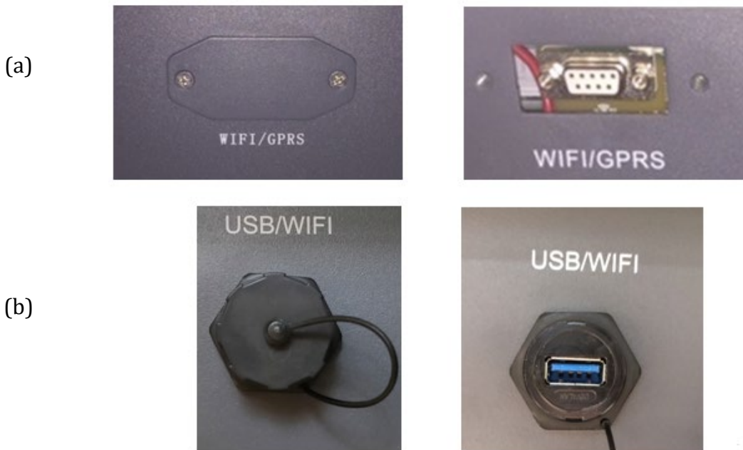
Figure 103 - Slot for external Wi-Fi adapter
