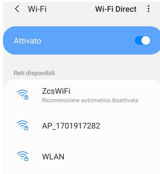
Figure 153 - Disabling automatic reconnection to a network
