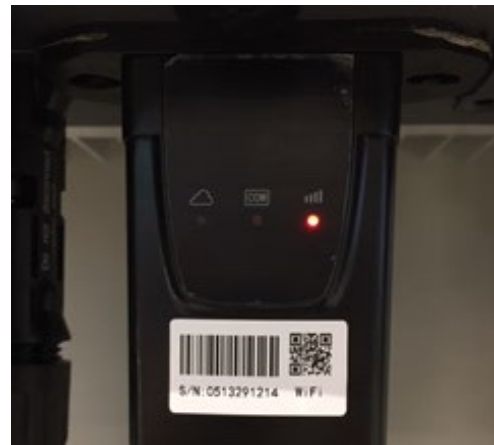
Figure 124 – Irregular communication status between Wi-Fi and remote server
