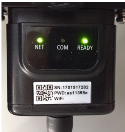
Figure 122 - Irregular communication status between inverter and Wi-Fi
