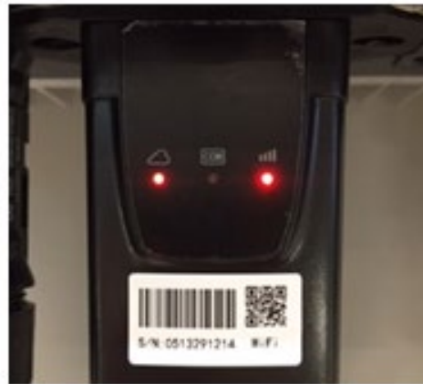
Figure 122 - Irregular communication status between inverter and Wi-Fi
