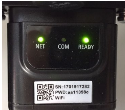
Figure 133 - Irregular communication status between inverter and adapter
