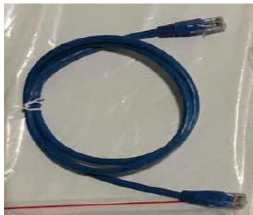
Figure 76 – Communication cable between AZZURRO 5000 PRO batteries
