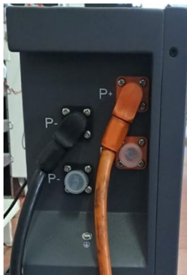
Figure 82 – Terminal block of the AZZURRO ZSX 5120 battery
