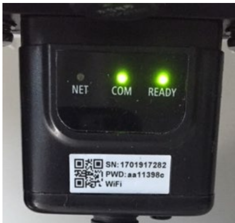
Figure 124 – Irregular communication status between Wi-Fi and remote server
