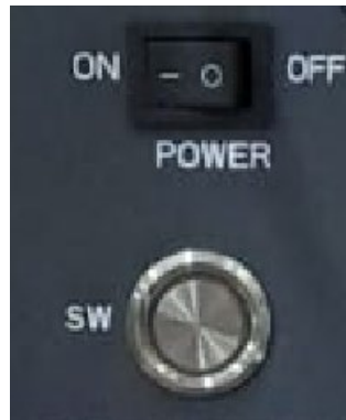
Figure 83- Power button of the AZZURRO ZSX 5120 battery
