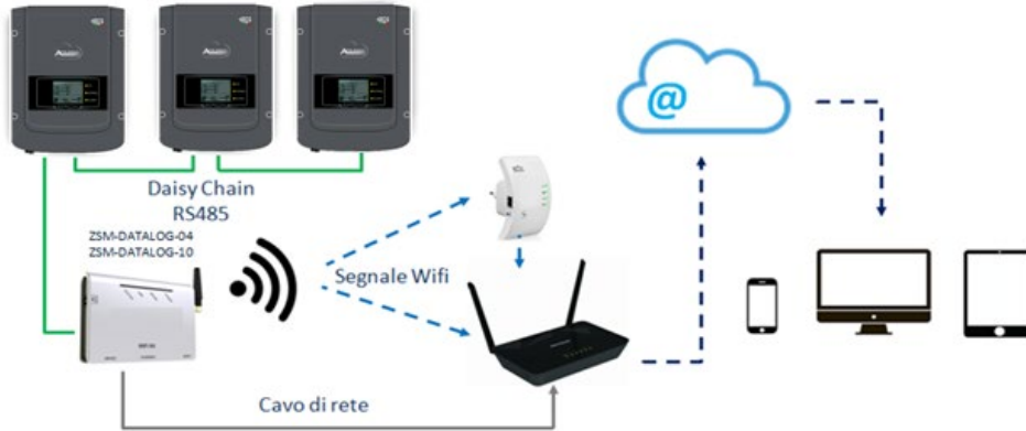
Figure 141 – Diagram for connecting the ZSM-DATALOG-04 / ZSM-DATALOG-10 datalogger
