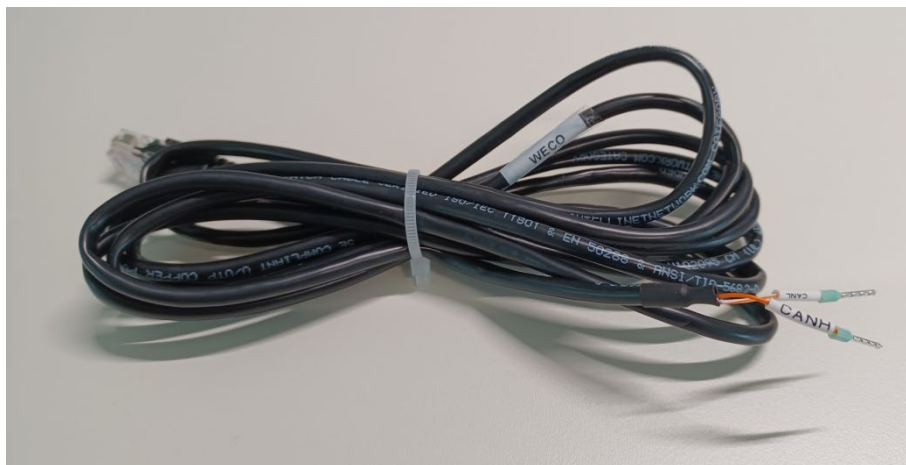
Figure 53 - Communication cable between the inverter and WeCo 5K3XP battery
