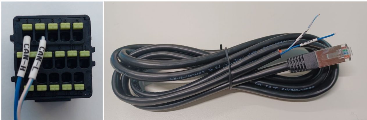
Figure 16 - Pylontech communication cable to be inserted into the battery communication input
