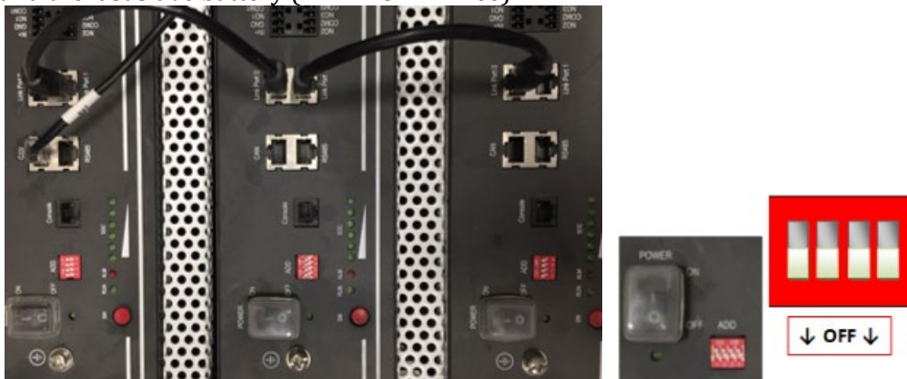
Figure 14- Connecting the communication cable between three Pylontech batteries
