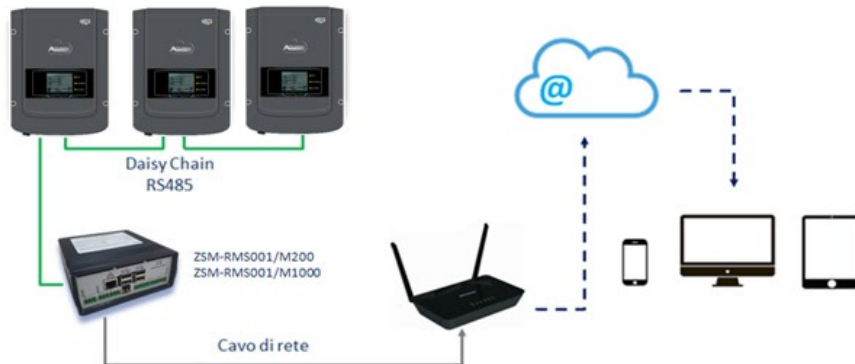
Figure 142 – Diagram for the functioning of the ZSM-RMS001/ M200 / ZSM-RMS001/M1000 datalogger
