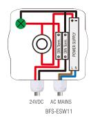
Using appropriate fixings attach the BFS-ESW11 unit vertically to the chosen surface.
