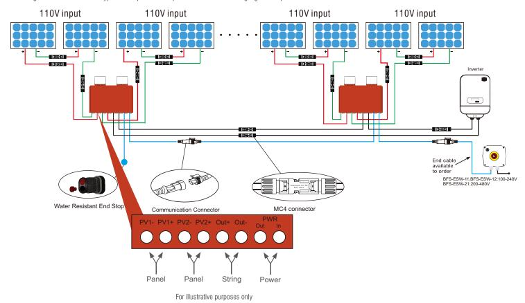
If the array has an odd number of panels, a single panel can be connected directly to the positive (+) and negative (-) panel cables of the BFS.
