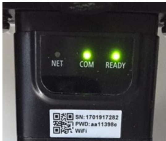
Figure 116 - Irregular communication status between the adapter and remote server
