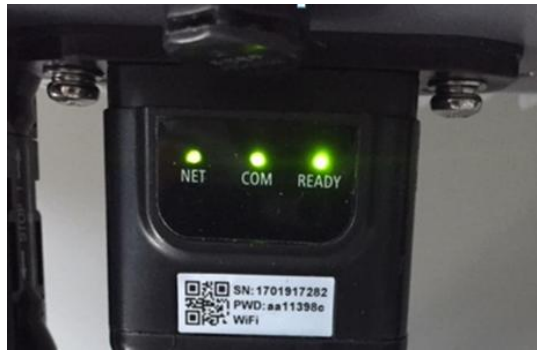
Figure 120 - Final status of LEDs
