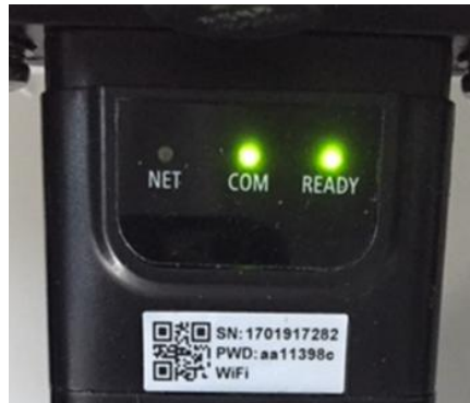
Figure 122 - Irregular communication status between the adapter and remote server
