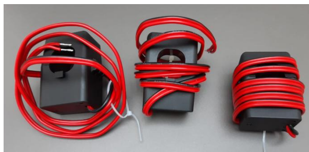
Figure 68 - Meter (top), CT sensors (low)
