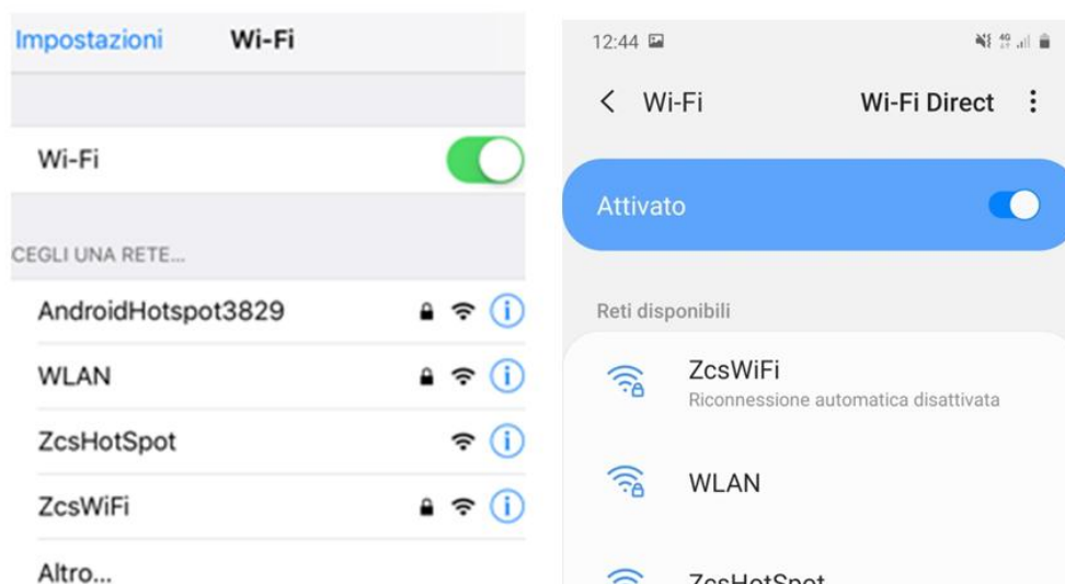
Figure 72 - Wi-Fi network search on Smartphone (iOS and Android); Access point of the Wi-Fi adapter is no longer visible
