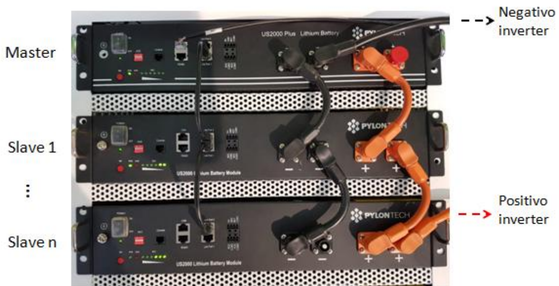
Figure 11 - Connecting three Pylontech batteries in parallel
