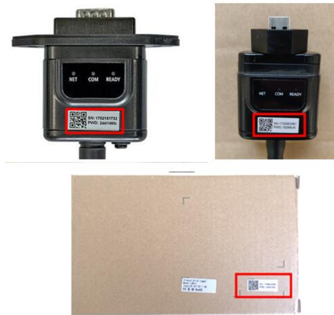
Figure 62 – Password of external Wi-Fi adapter
