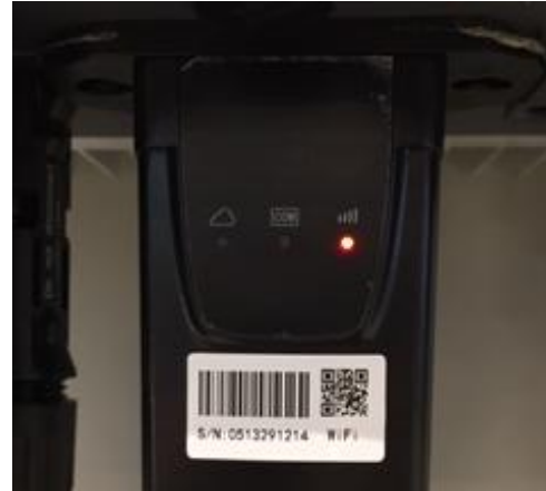
Figure 79 - Irregular communication status between Wi-Fi and remote server
