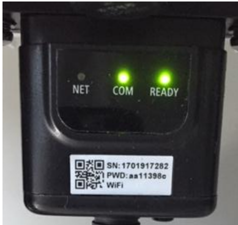
Figure 79 - Irregular communication status between Wi-Fi and remote server
