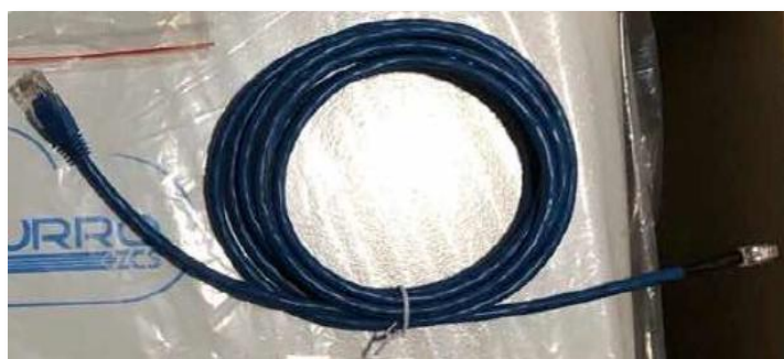
Figure 15 - Communication cable between the inverter and WeCo battery
