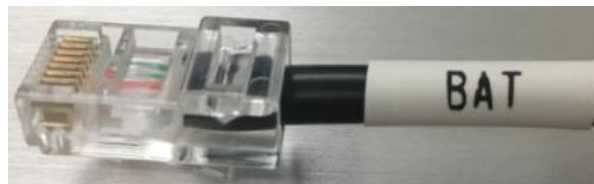
Figure 11 - Pylontech communication cable to be inserted into the battery communication input
