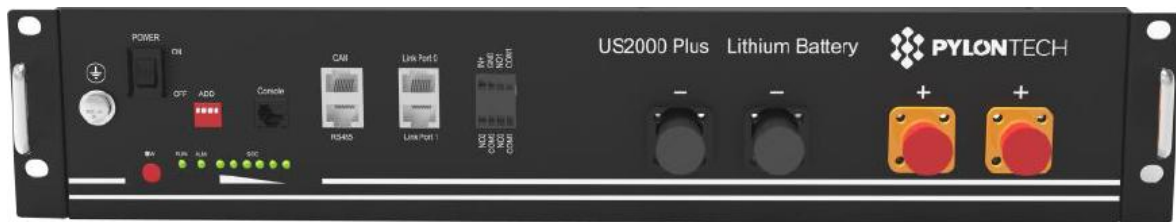
Figure 50 – Battery status after setting the POWER switch to ON and pressing the SW button
