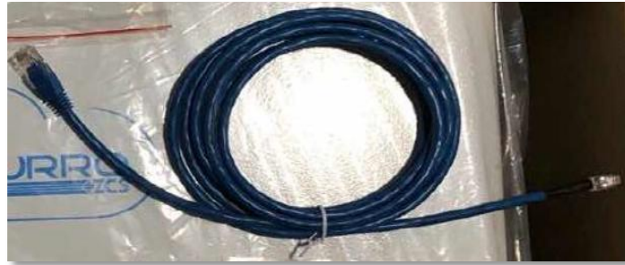
Figure 12 - Communication cable between the inverter and WeCo battery
