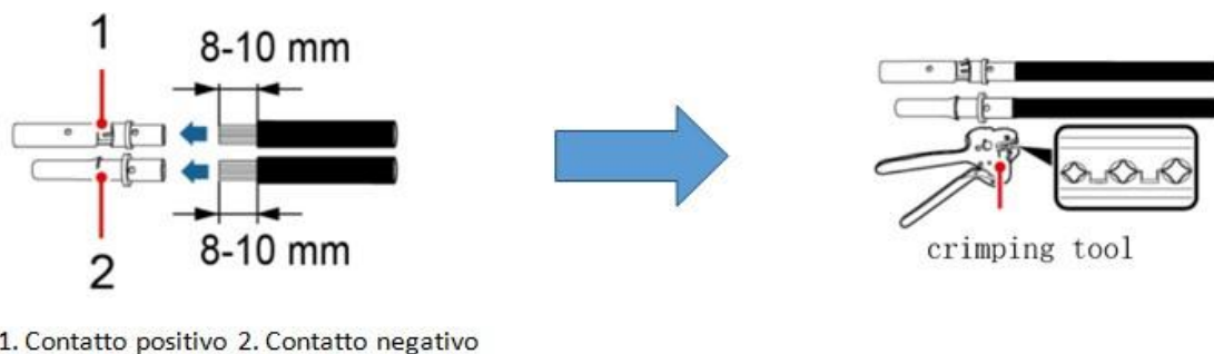
Figure 19 - Preparing the positive and negative photovoltaic cables
