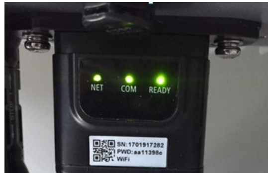
Figure 76 - Final status of LEDs
