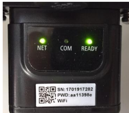
Figure 77 - Irregular communication status between inverter and adapter
