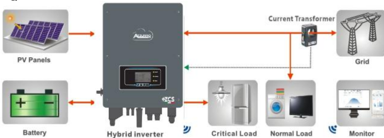
Figure 1 - Diagram of a system on which a 1PH HYD3000-HYD6000-ZSS hybrid is installed
