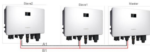
Figure 1-2 Master-slave inverter communication wiring
